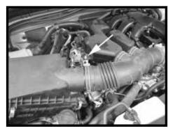
Step 5 Remove the mounting screw which holds the intake tube to the bracket.
