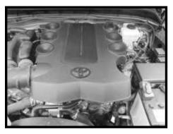
Step 2 Remove the engine cover.
