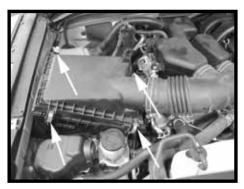
Step 7 Unclip the four hold down clips on the air filter lid. Remove the air filter lid/intake tube assembly and air filter.
