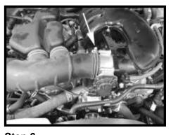
Step 6 Loosen the clamp at the throttle body.
