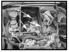
Step 8 Loosen the three bolts and remove the lower air box from the vehicle.
