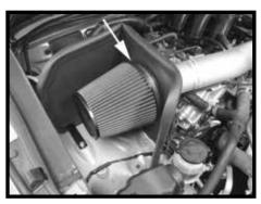
Step 19 Install air filter with the supplied clamp and fully tighten.
