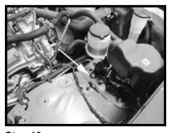
Step 13 Remove the bolt that secures the power steering reservoir. This bolt will be re installed with the new heat shield.
