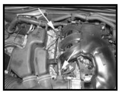
Step 3 Disconnect the fuel pressure vent line from the fuel pressure regulator and the crank case vent line.
